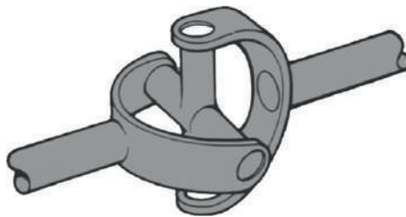
Figure 5.84 Detail of a universal joint
